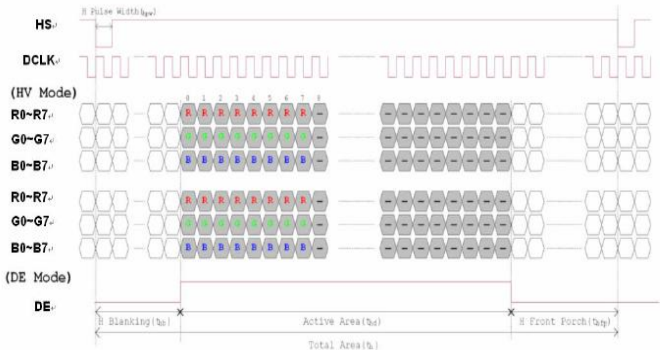
Figure 3. 1 Horizontal input timing diagram.
